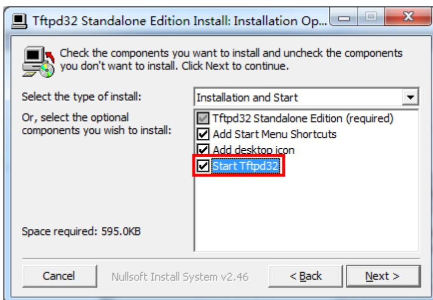
Select **Start Tftpd32** (marked in red box in the screen capture above), and then click the **Next** button and follow the on-screen instructions to complete the installation.
