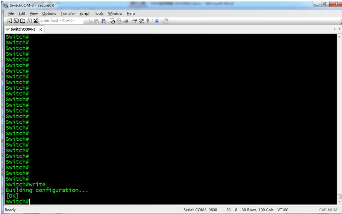
Now, it has successfully saved configuration used in single switch networking. Switch will run this configuration for the next startup.
