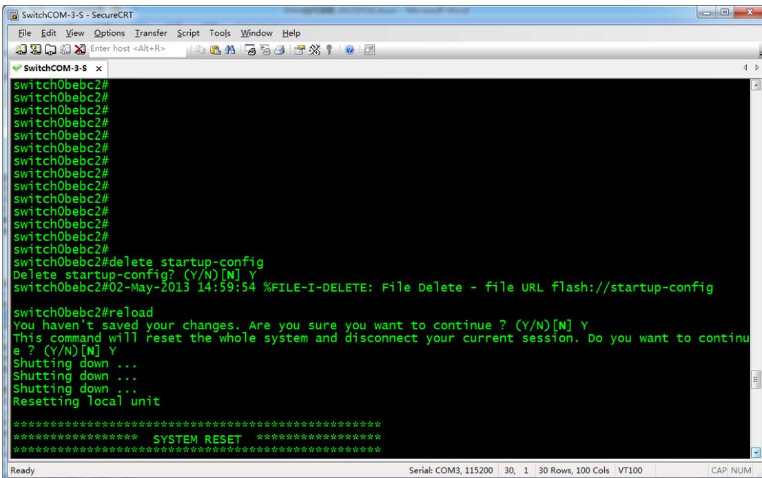
3. Switch reboots. When the following prompt appears, quickly press **Enter** twice to complete the baud-rate detection process.
