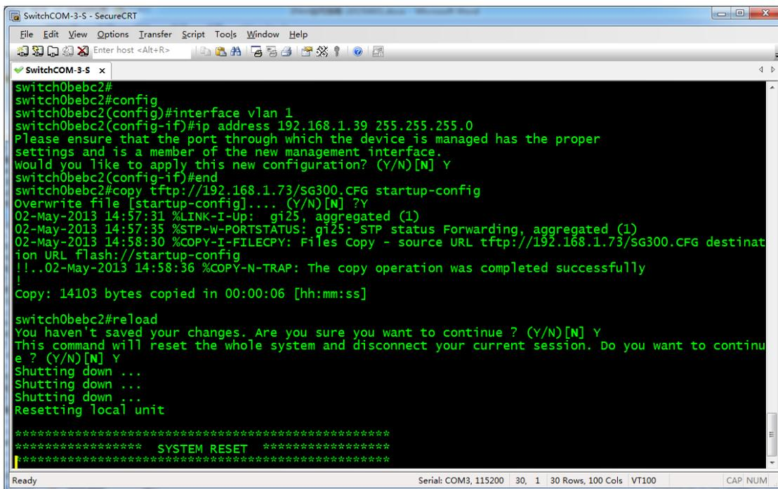
After rebooting, switch runs configuration file **SG300.CFG**.
