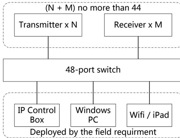
Above is a topology of a single 48-port 1000Mbps Ethernet switch. We recommend:
