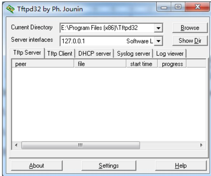
You need to configure **Current Directory** and **Server interfaces** before using **tftpd32** to perform import and export configuration for switches.
