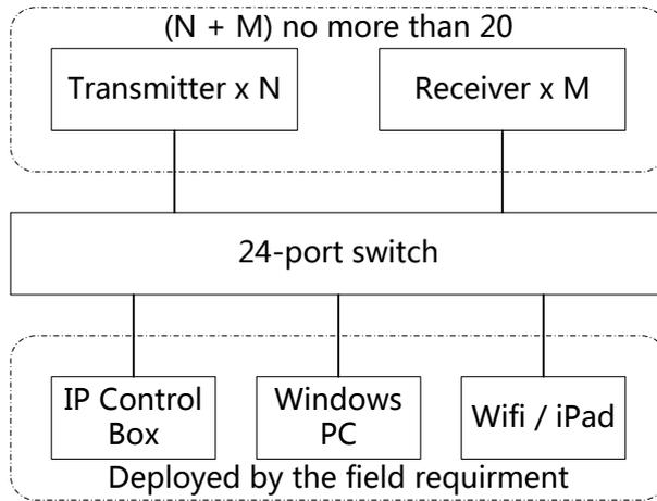
Above is a topology of a single 24-port 1000Mbps Ethernet switch. We recommend:
